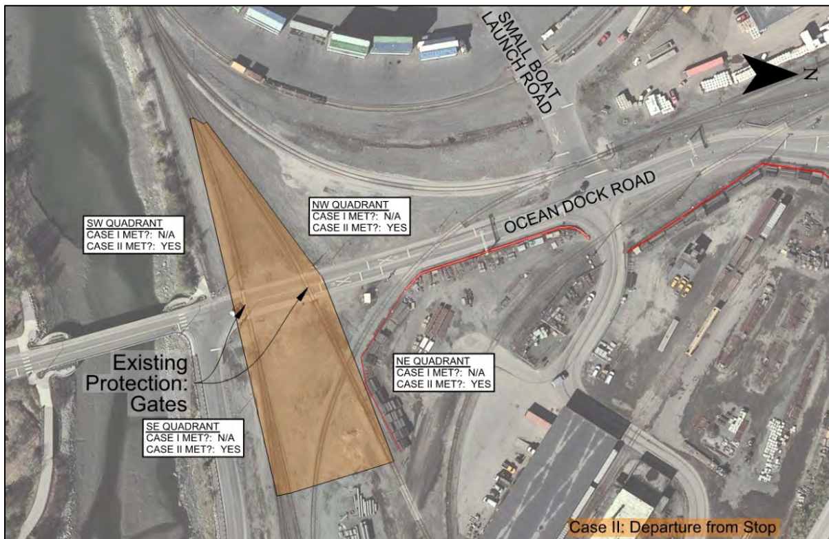
Figure 22: Rail-Road Ocean Dock Road 1 & 2 (868537M) Crossing Sight Triangles
