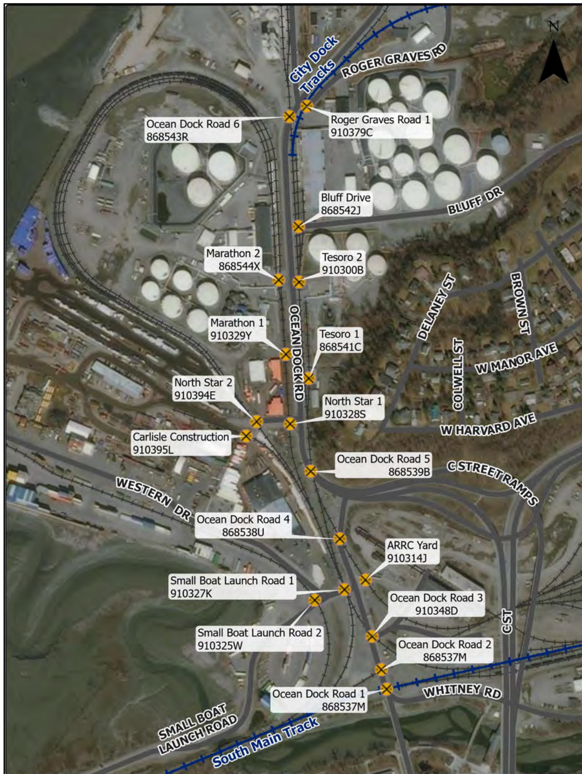
Figure 20: Rail-Road At-Grade Crossing Locations
