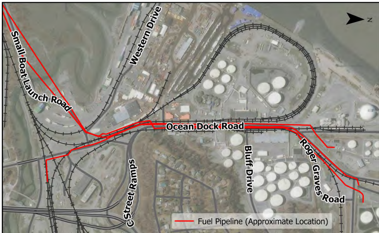
Figure 12: Study Area Fuel Pipelines
