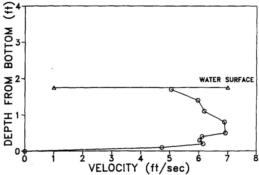
Figure 33. Water velocity profile, culvert outlet, 21 May 1986.
