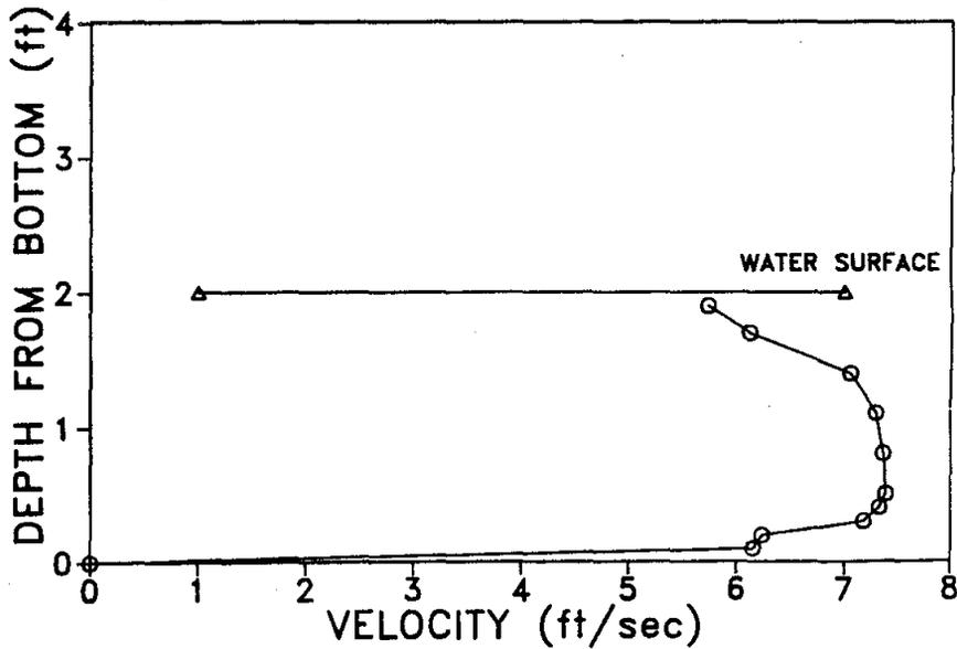
Figure 18. Water velocity profile, culvert outlet, 18 May 1986.
