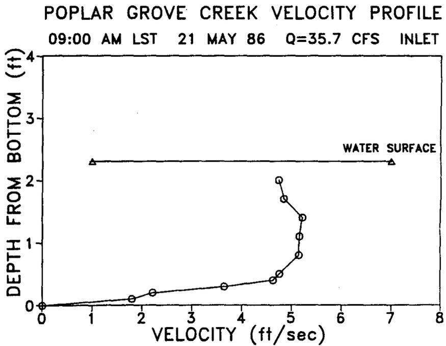
Figure 30. Water velocity profile, culvert inlet, 21 May 1986.
