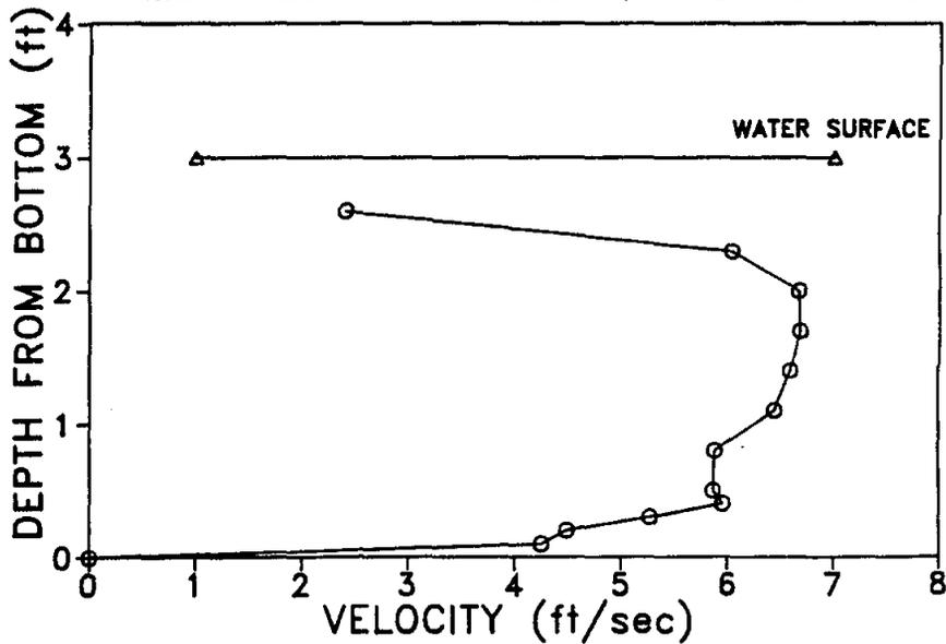
Figure 12. Water velocity profile, 1.2 m downstream culvert inlet, 16 May 1986.
