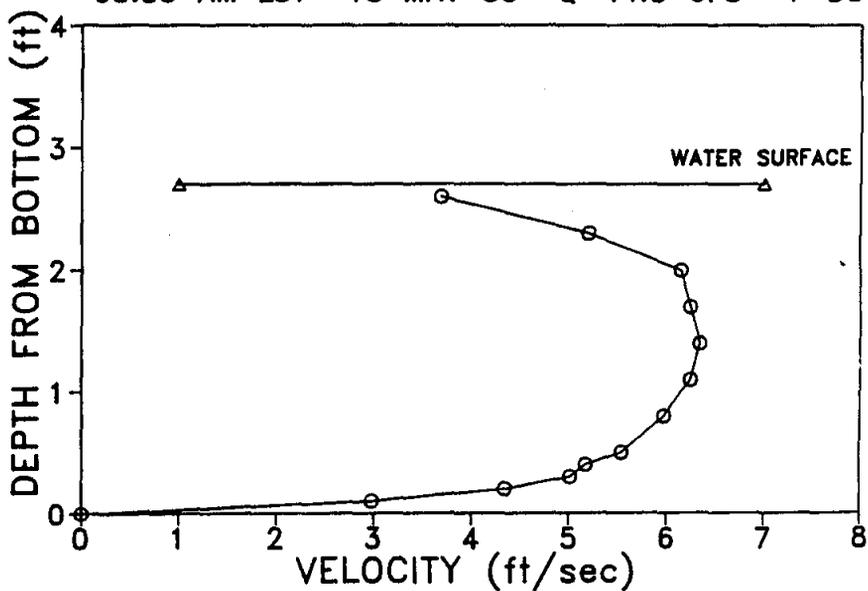
Figure 16. Water velocity profile, 1.2 m downstream culvert inlet, 18 May 1986.
