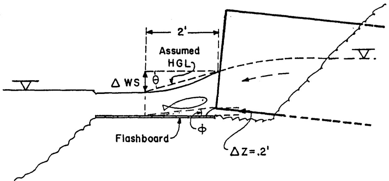
Figure 54. Culvert outlet conditions encountered by fish migrating upstream.
