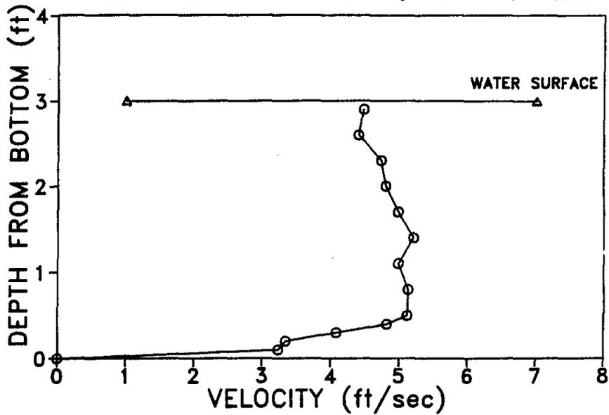
Figure 11. Water velocity profile, culvert inlet, 16 May 1986.
