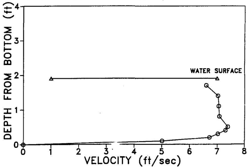
Figure 23. Water velocity profile, culvert outlet, 19 May 1986.
