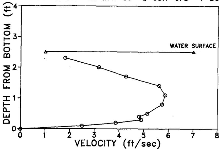
Figure 31. Water velocity profile, 1.2 m downstream culvert inlet, 21 May 1986.
