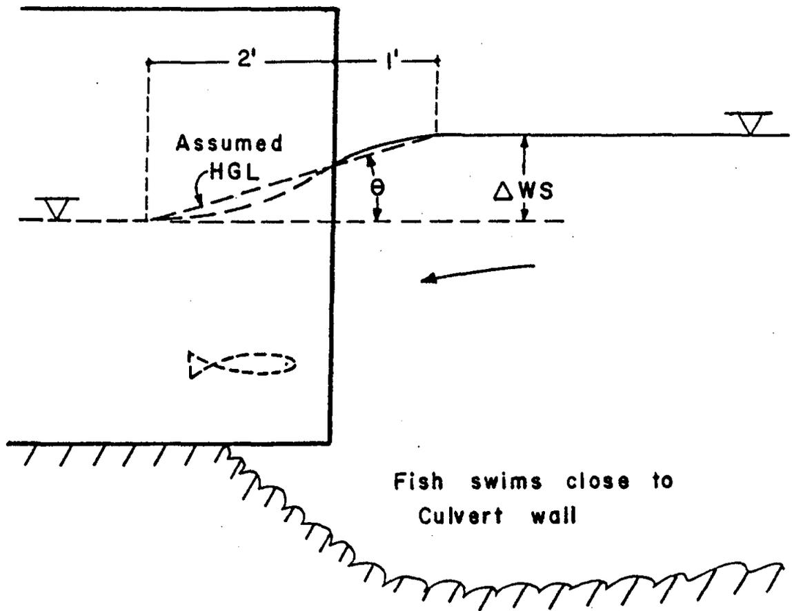
Figure 55. Culvert inlet conditions encountered by fish migrating upstream.
