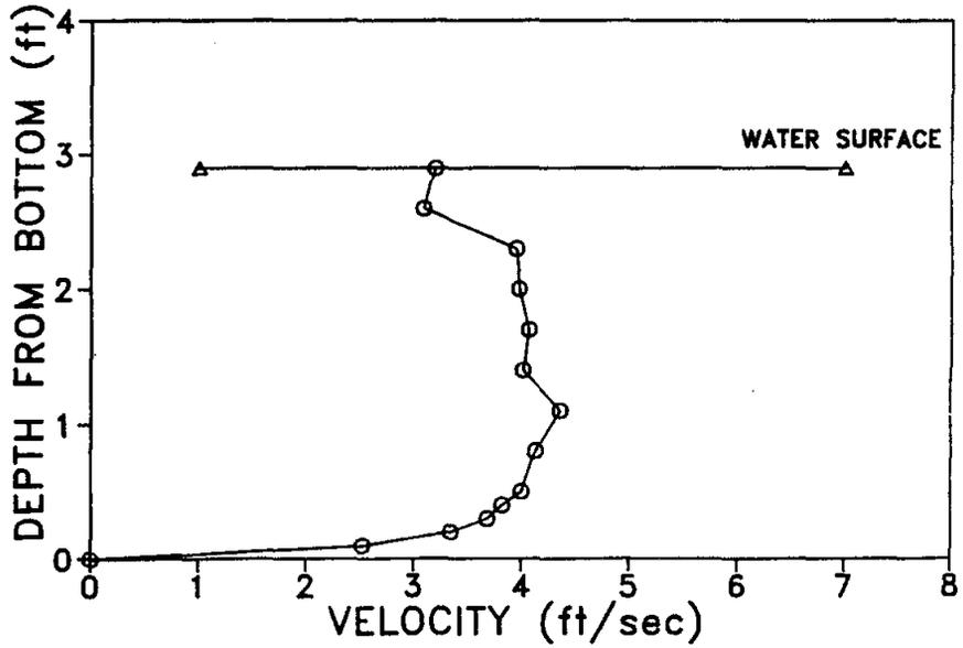
Figure 22. Water velocity profile, 1.5 m upstream culvert outlet, 19 May 1986.
