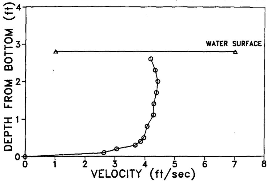
Figure 27. Water velocity profile, 1.5 m upstream culvert outlet, 20 May 1986.
