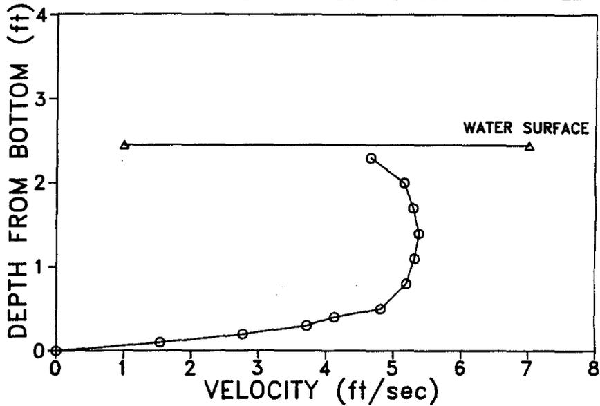
Figure 25. Water velocity profile, culvert inlet, 20 May 1986.
