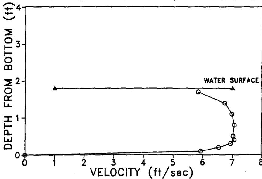
Figure 28. Water velocity profile, culvert outlet, 20 May 1986.
