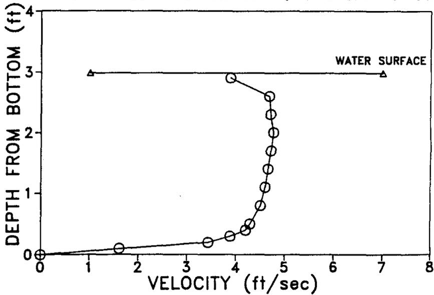
Figure 17. Water velocity profile, 1.5 m upstream culvert outlet, 18 May 1986.
