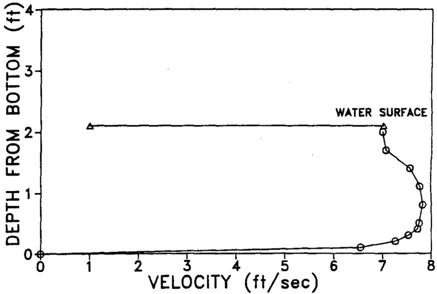
Figure 14. Water velocity profile, culvert outlet, 16 May 1986.
