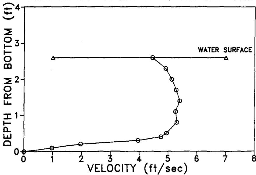
Figure 20. Water velocity profile, culvert inlet, 19 May 1986.
