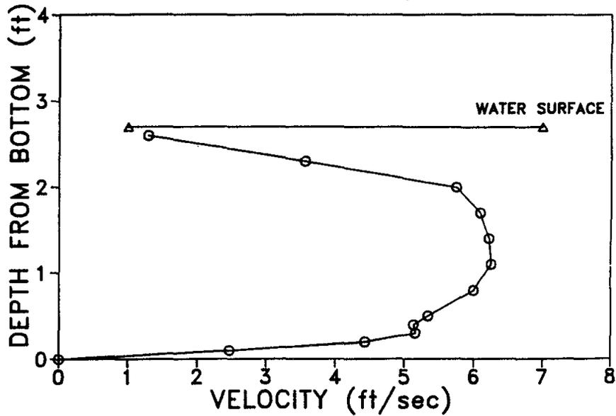
Figure 21. Water velocity profile, 1.2 m downstream culvert inlet, 19 May 1986.
