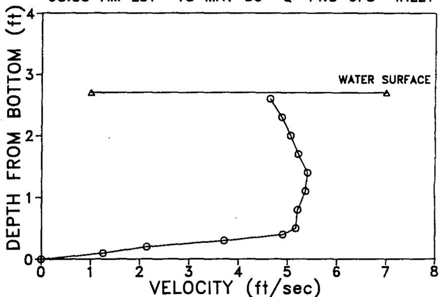
Figure 15. Water velocity profile, culvert inlet, 18 May 1986.
