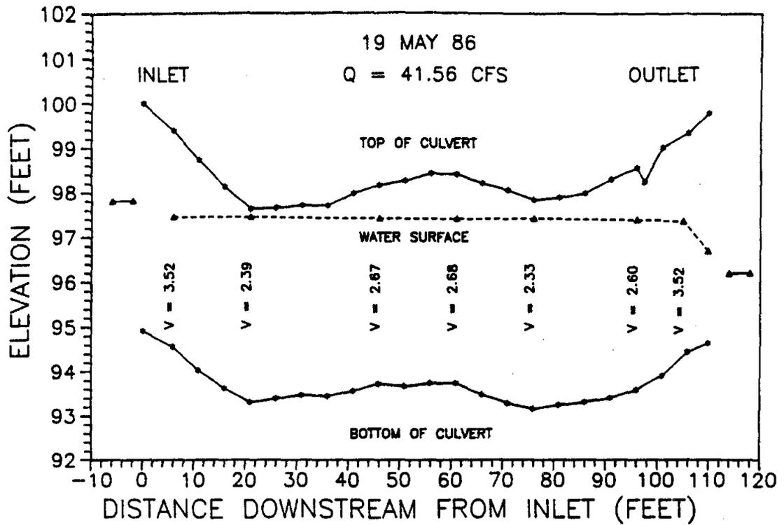
Figure 37. Calculated culvert water surface profiles, 19 May 1986.
