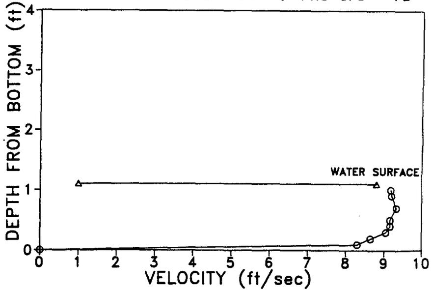
Figure 19. Water velocity profile, outlet flash board, 18 May 1986.
