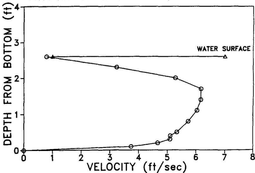
Figure 26. Water velocity profile, 1.2 m downstream culvert inlet, 20 May 1986.
