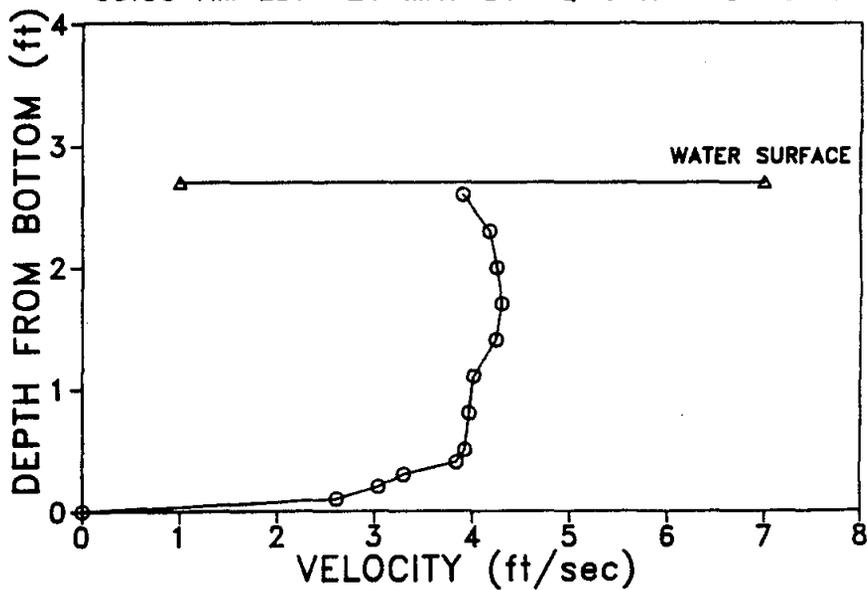
Figure 32. Water velocity profile, 1.5 m upstream culvert outlet, 21 May 1986.
