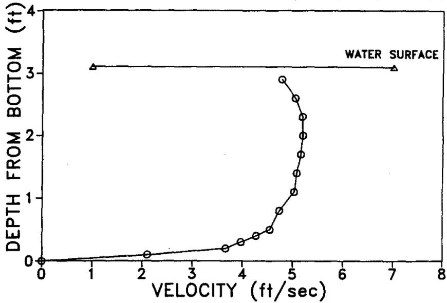
Figure 13. Water velocity profile, 1.5 m upstream culvert outlet, 16 May 1986.
