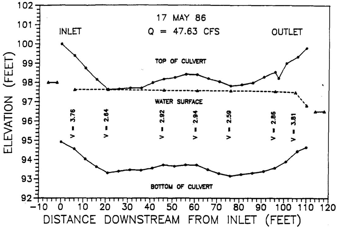
Figure 35. Calculated culvert water surface profiles, 17 May 1986.
