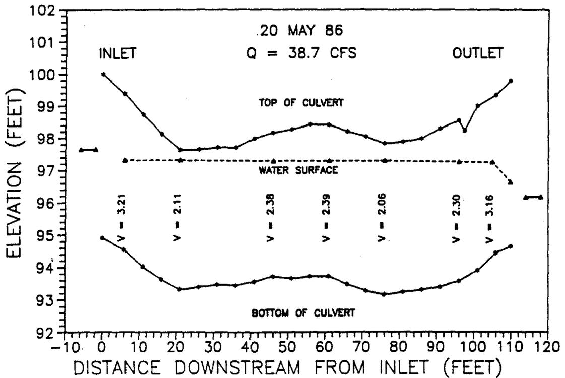
Figure 38. Calculated culvert water surface profiles, 20 May 1986.
