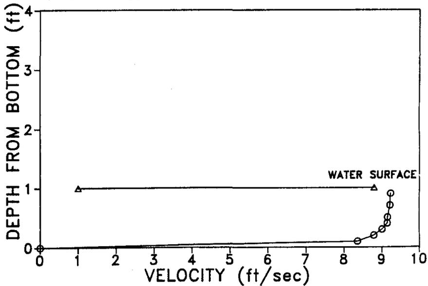
Figure 24. Water velocity profile, outlet flash board, 19 May 1986.
