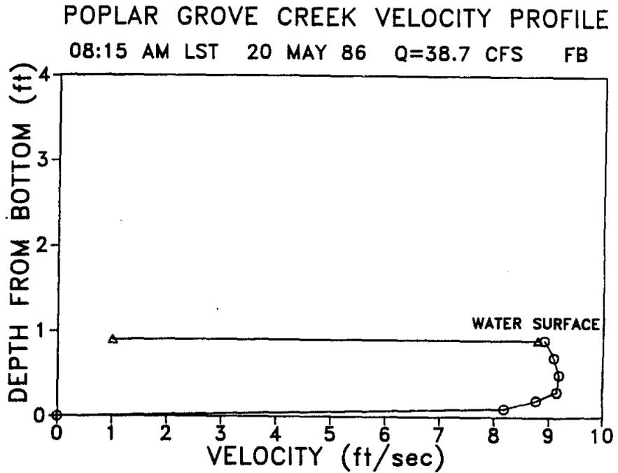
Figure 29. Water velocity profile, outlet flash board, 20 May 1986.
