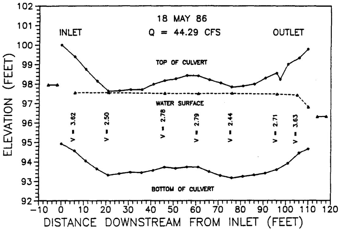
Figure 36. Calculated culvert water surface profiles, 18 May 1986.
