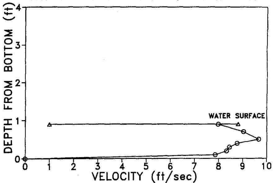
Figure 34. Water velocity profile, outlet flash board, 21 May 1986.
