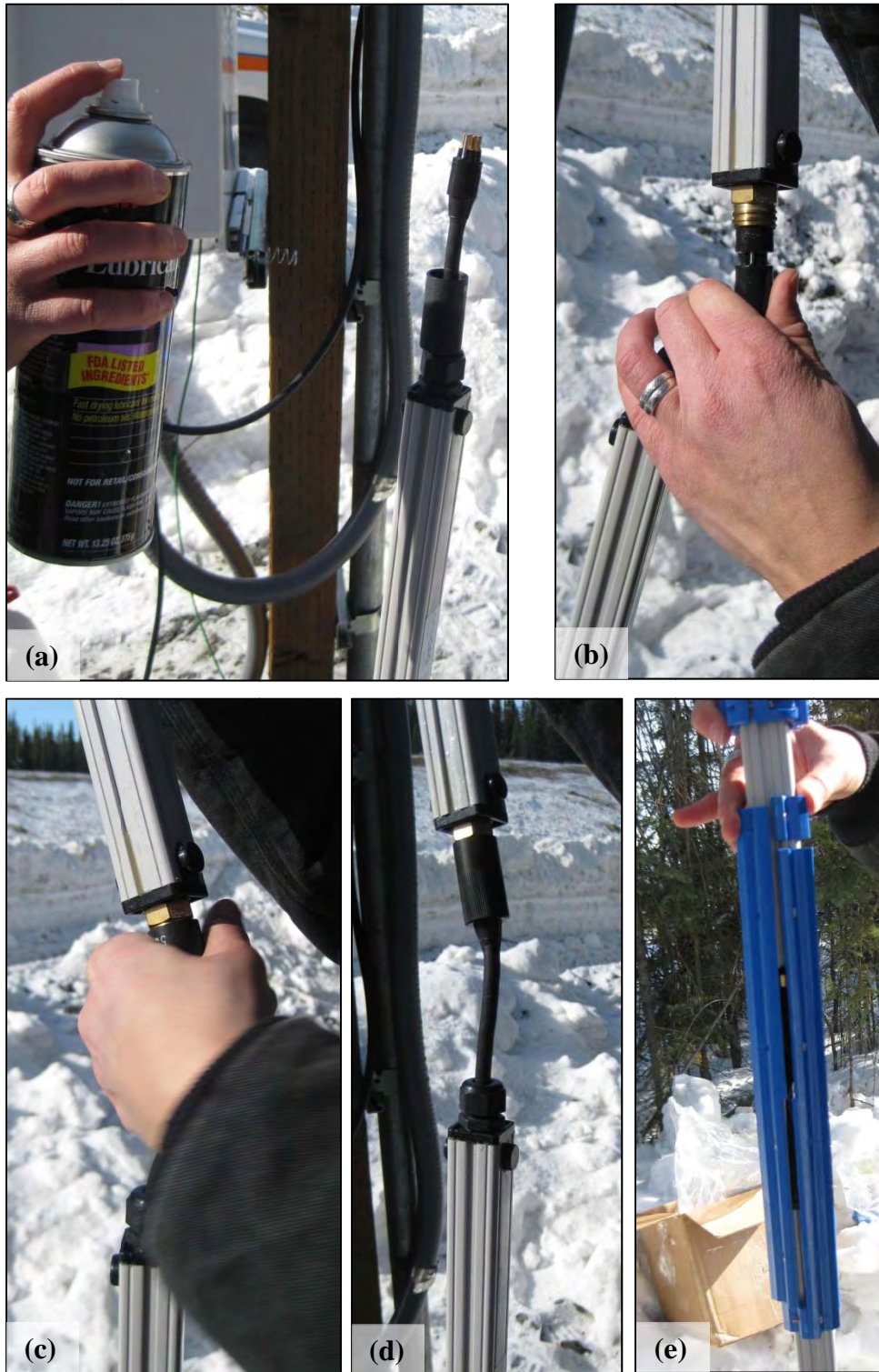
Figure A-11. Steps in the assembly of the INC500 modules. (a) Spraying the connections with silicon; (b) plugging the water-tight connectors together; (c) screwing the threaded connections together for the water-tight connection; (d) connected modules; (e) attaching the coupler assembly. (Photographs courtesy of A. Parsons, March 2010)
