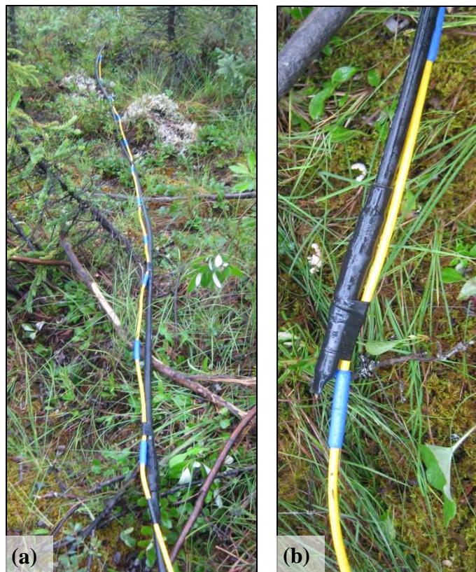
Figure C-6. Alignment of TAC and thermistor cable. (a) Location of thermistor beads relative to TAC sensors was recorded, (b) as well as the location of the final thermistor bead. (Photographs by M. Darrow, July 2012)
