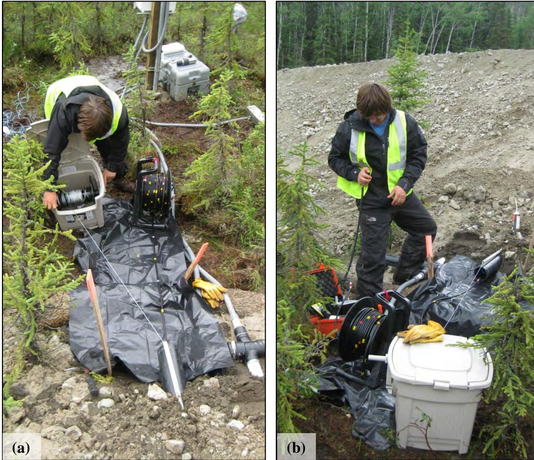
Figure C-22. Taking manual inclinometer probe measurements. (a) Feeding inclinometer probe cable into casing by reeling up the wire rope; (c) taking readings as the cable is retracted from the casing. (Photographs by M. Darrow, July 2012)
