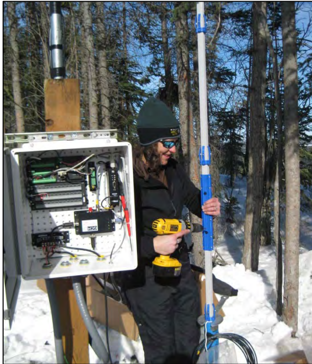
Figure A-12. Connecting the coupler assembly with machine screws. (Photograph courtesy of A. Parsons, March 2010)
