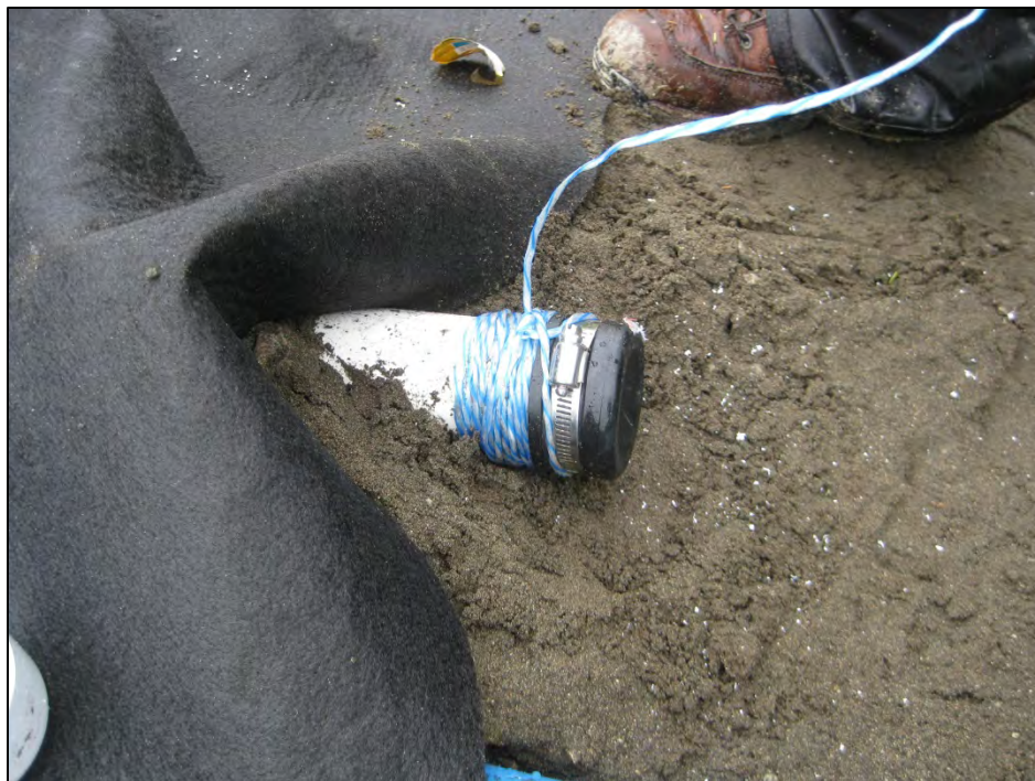
Figure C-8. Uphill termination of the casing containing the TAC and thermistor string. (Photograph by M. Darrow, July 2012)
