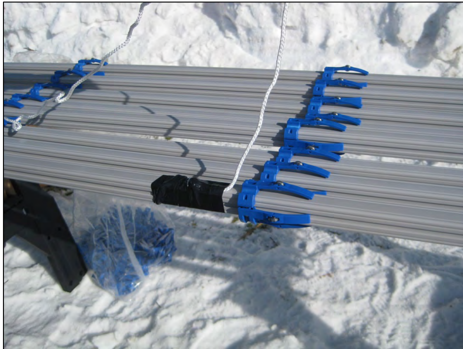
Figure A-8. Attaching the safety line to the lowest module. (Photograph by M. Darrow, March 2010)
