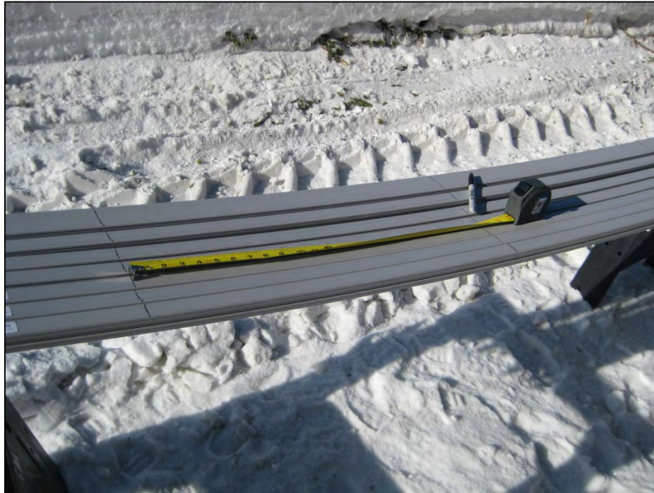
Figure A-5. Marking the INC500 for placement of centralizers. (Photograph by M. Darrow, March 2010)
