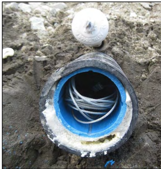
Figure C-23. Downslope guide casing termination. Wire rope is tucked into casing for easy retrieval for next reading. (Photographs by M. Darrow, July 2012)
