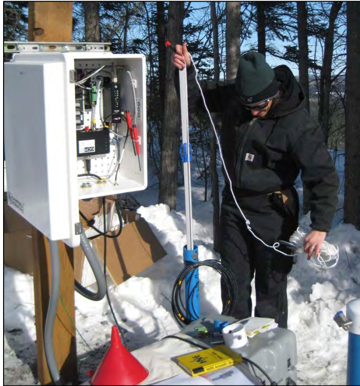
Figure A-9. Lowering the first INC500 module down the guide casing. (Photograph courtesy of A. Parsons, March 2010)
