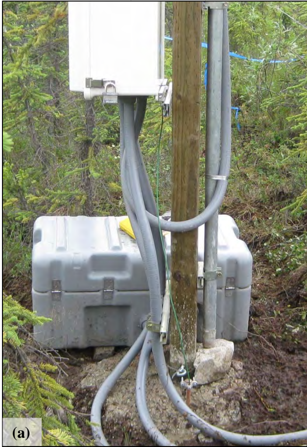
Figure C-28. Changes at the ADAS during the fall of 2012. (a) Post, solar panel support, and grounding rod on July 11, 2012; (b) Settlement of ground surface as of October 6, 2012. (Photographs by M. Darrow and D. Jensen)
