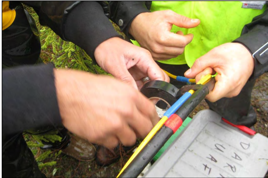
Figure C-5. Wrapping BeadedStream temperature acquisition cable (TAC) to thermistor cable for installation. (Photograph by M. Darrow, July 2012)
