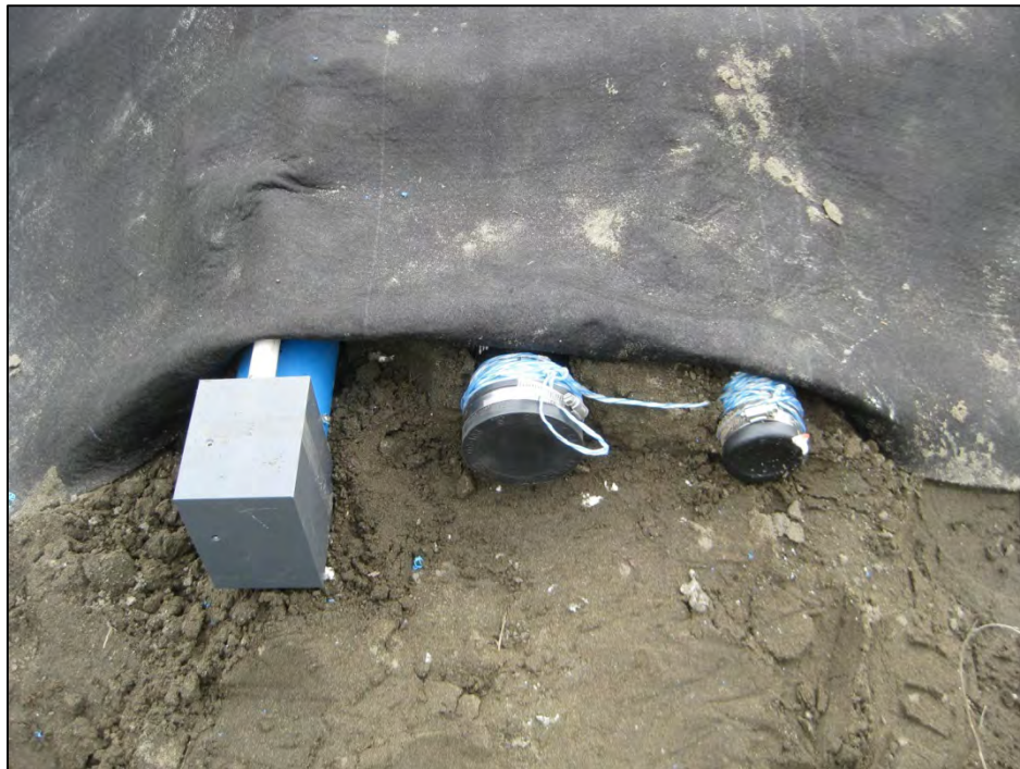
Figure C-17. Upslope casing ends secured. From left to right, dead-end pulley on guide casing for manual inclinometer probe measurements, sealed guide casing with tied-off SAA pull rope, sealed 2-in. PVC casing with tied-off TAC/thermistors string pull rope. (Photograph by M. Darrow, July 2012)
