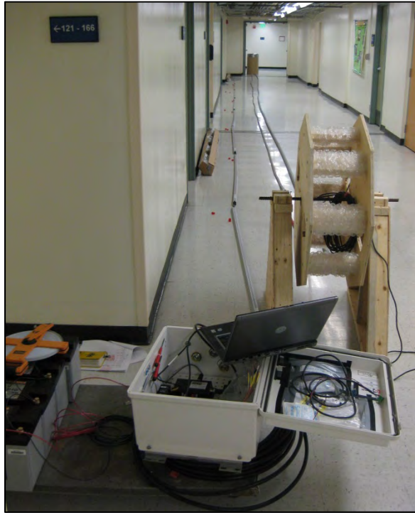
Figure A-3. Conducting a “hallway” test with the INC500 and SAA devices wired into the ADAS enclosure. (Photograph by M. Darrow, March 2010)
