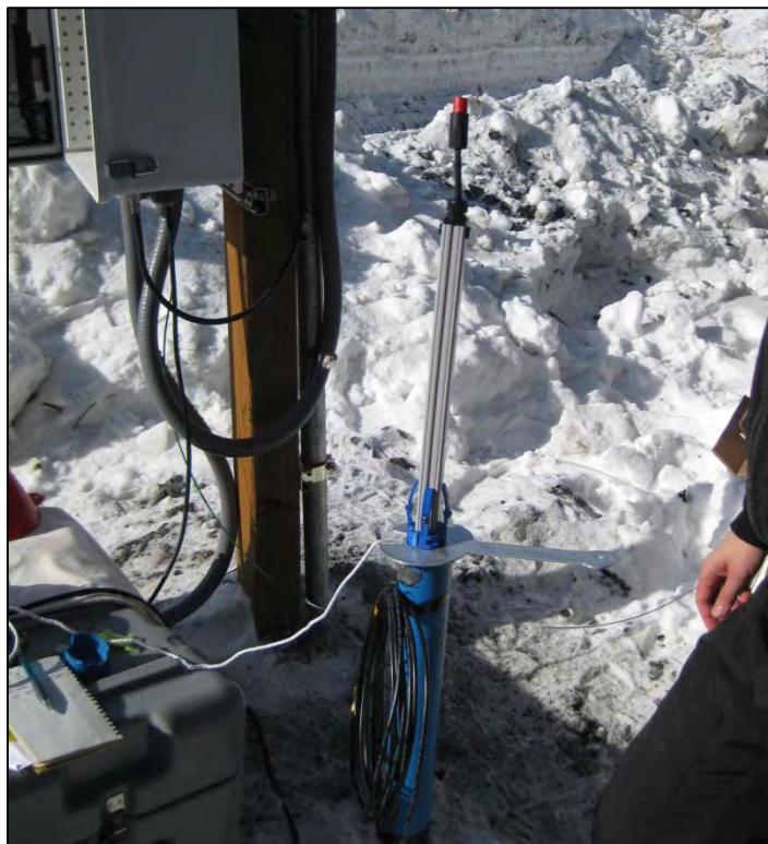
Figure A-10. First INC500 module resting on fork. (Photograph courtesy of A. Parsons, March 2010)
