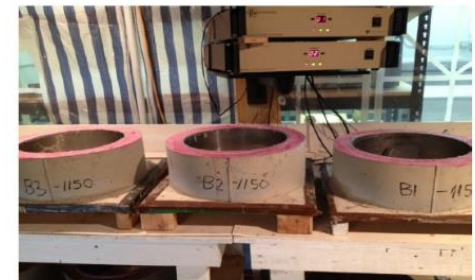
Mix 2013-010 (ASTM C1581 @ 24 Hours) Accelerated Portland Cement Samples
