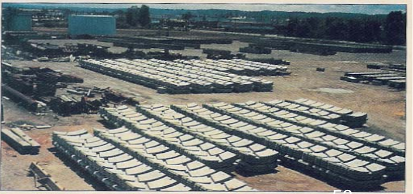
Part of the 16,000 precast liner segments supplied to the bus tunnel project by Concrete Technology Corp.
