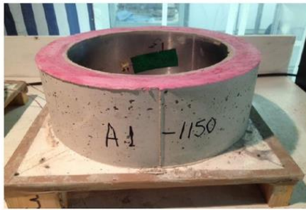
Mix 2013-009 (No Cracking at 90 Days)
