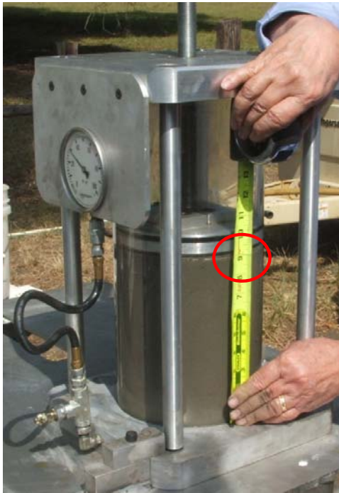
At 30 psi pressure, the cellular concrete was reduced in height to 9 inches
