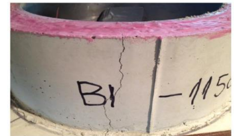
Mix 2013-010 (Cracked at 7.94 Days)
