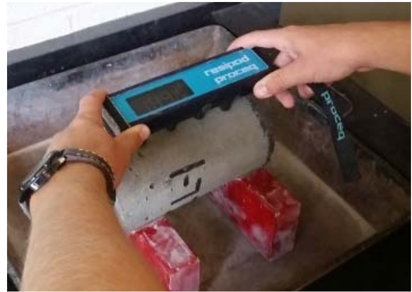
Resistivity testing for mixture acceptance
