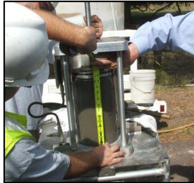
The cellular concrete level was 12 inches at zero pressure
