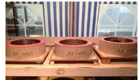
Mix 2013-009 (ASTM C1581 @ 24 Hours) Belitic CSA Cement Samples
