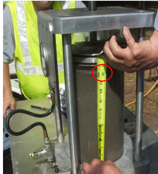
*Note there was no visible collapse of the cellular concrete after the test.
