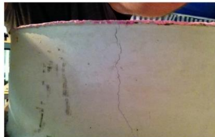
Mix 2013-010 (Cracked at 9.54 Days)
