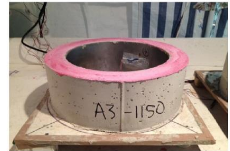
Mix 2013-009 (No Cracking at 90 Days)
