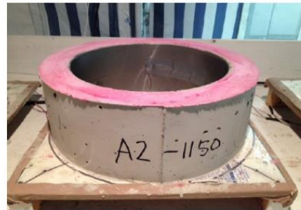
Mix 2013-009 (No Cracking at 90 Days)
