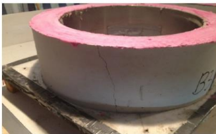
Mix 2013-010 (Cracked at 9.21 Days)
