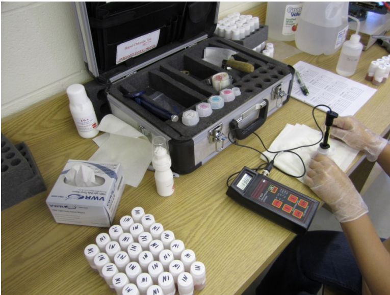
Drilled powder samples tested for chloride content
