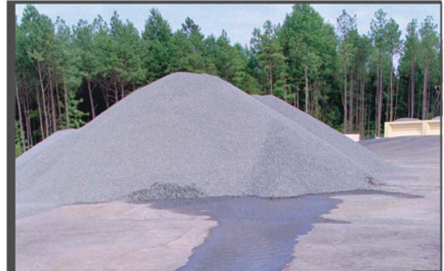
WATER DRAINS FROM SLOPED STOCKPILE
