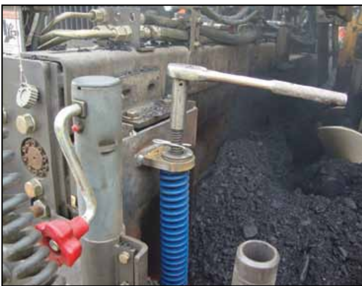
Floating cotter pin for engaging and disengaging Safety Edge
