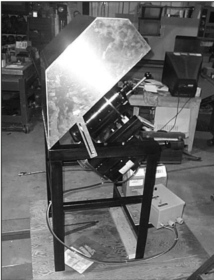
A new Nordic abrasion tester is fitted with a safety hood and is almost ready for delivery. You can see the drum is tilted in this picture. It can tip up for loading and down for unloading the sample charge.
