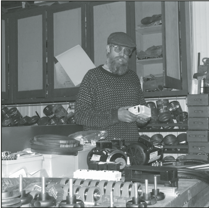
Jon Holmgren prepares a control unit for the Nordic abrasion testers. Parts for the testers are organized on the table in the foreground
