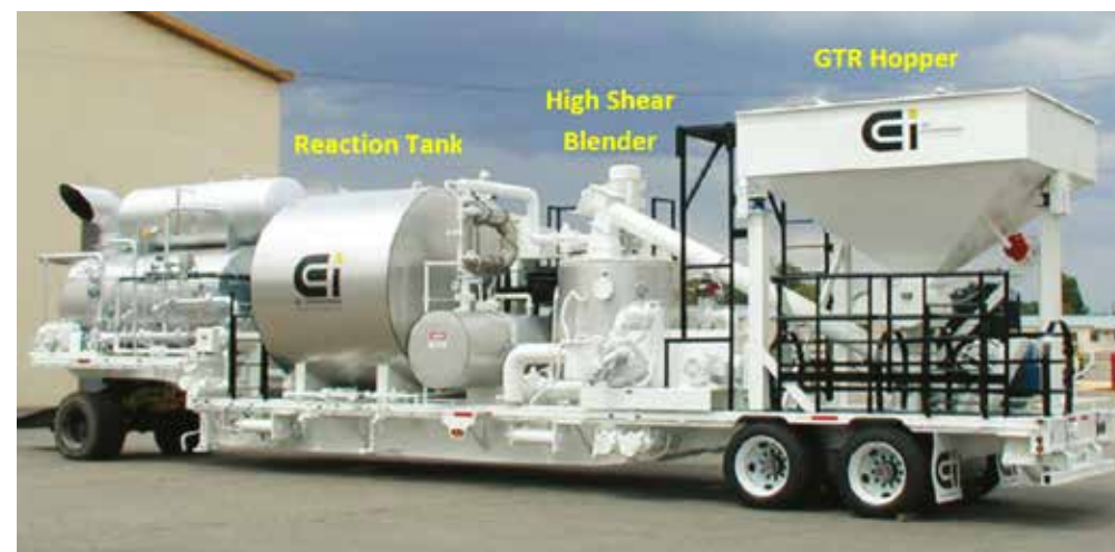
Asphalt Rubber Blending Unit
