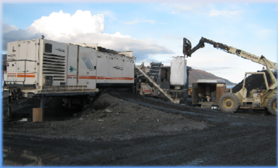
Wirtgen KMA 220 Mobile Plant
