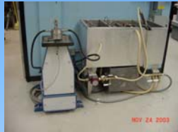
Prall Testing HMA Core To Simulate Studded Tire Wear
