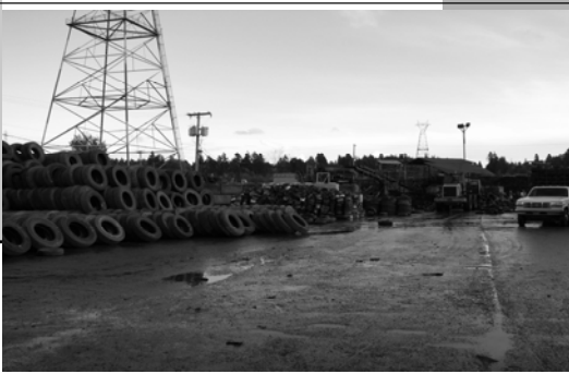
Western Rubber Co.: truck tires separated from light truck and car tires in receiving-initial processing yard
