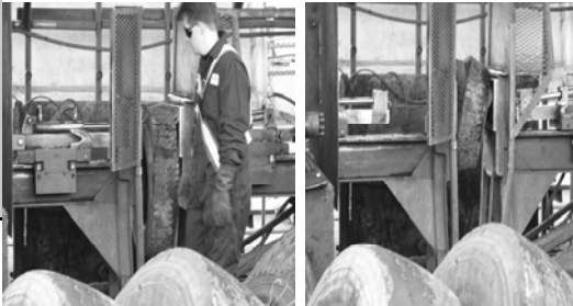
First steps - rip rim beads from tires, split in halves using a giant bagel slicer and stacked for processing. Very labor intensive production.
