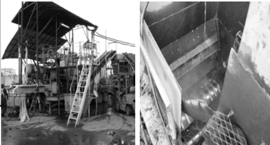
Shredding operation, two shredders process tire halves down to \pm 3 \times 8 inch chunks.
