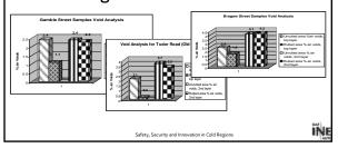
Wheel path voids increased in wheel path for SMA's except for Diamond.
