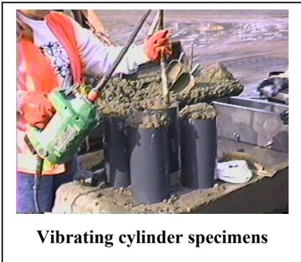
Vibrating cylinder specimens
