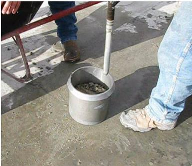
**Vibrating Concrete in Measure**
