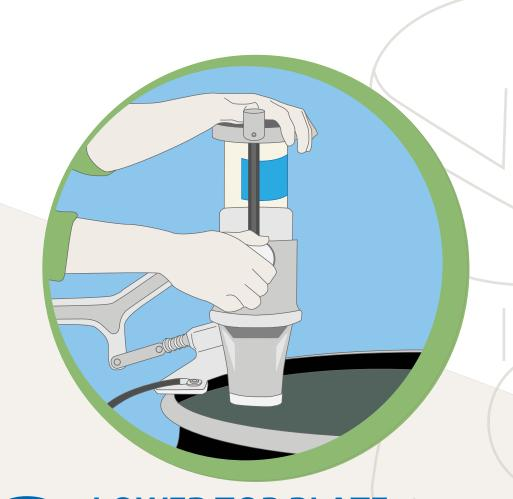
**LOWER TOP PLATE** Lower the sliding top plate and FIRMLY engage against plastic sleeve or bottom of "jumbo" can. TIGHTEN lock knob.
