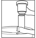
• Replace the entire Combination Filter every 9months, 2250 cans, or after the Activated Carbon Cartridge (upper portion) is changed-out twice. To replace simply
