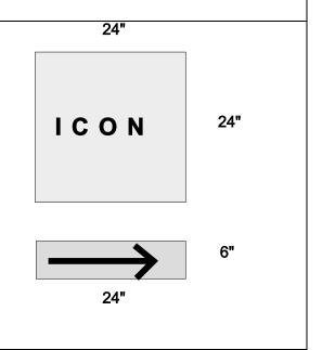
**Size of Signs**: The Trailblazing Signs consist of two signs; one sign measuring 24" by 24" and the other sign measuring 6" by 24". The 24" by 24" sign is located above the 6" by 24" sign on the same pole. Vertical spacing between the two signs shall be two inches. The sign panel thickness shall be 0.125 inches. All posts shall be 2 1/2 inch perforated steel tubes. All posts shall be installed in sleeve type concrete foundation.
