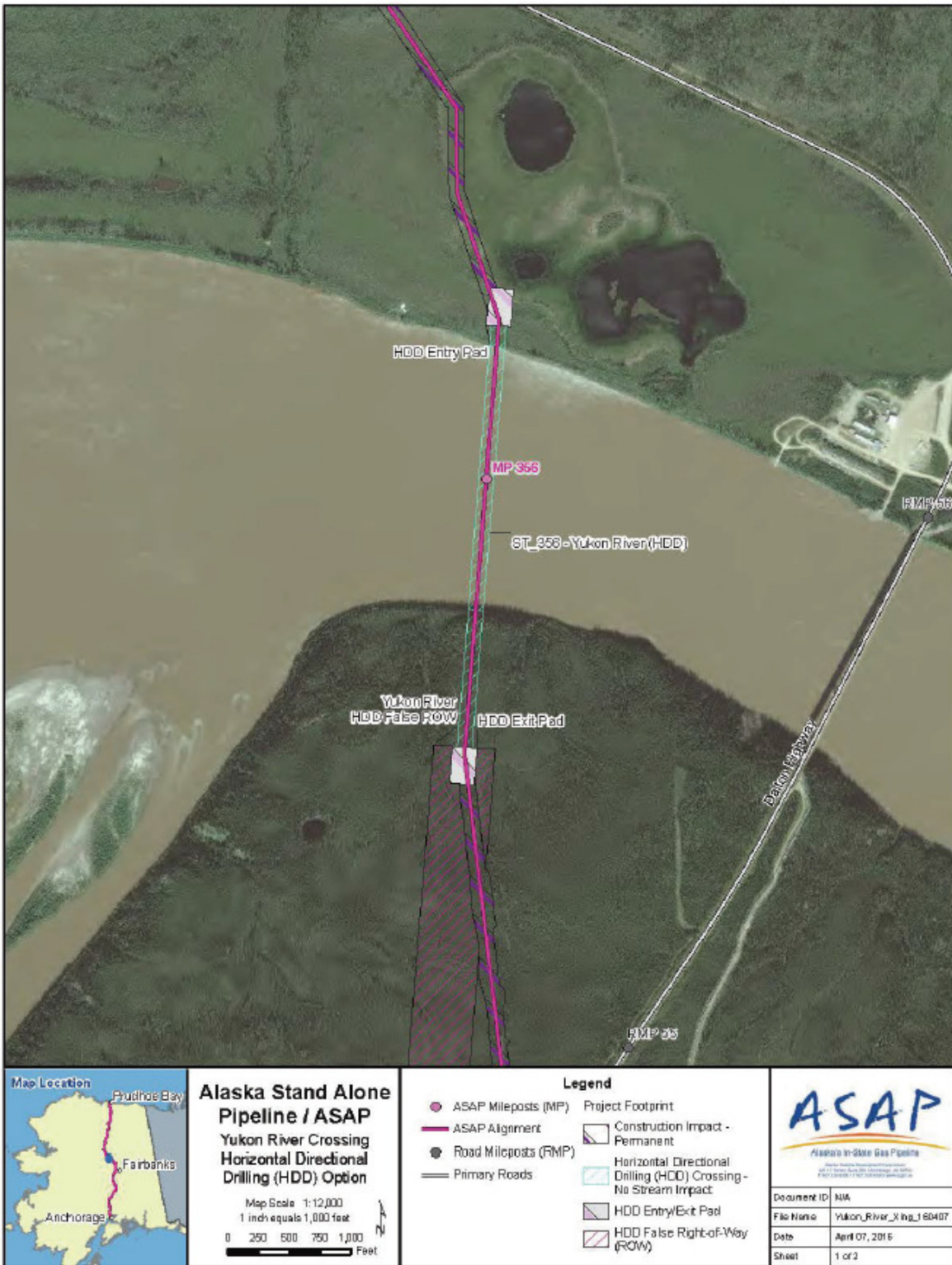
Figure 2-13. Alaska Stand Alone Gas Pipeline Proposed Pipeline Crossing of the Yukon River
