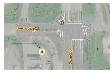
peak period. With the forecasted volumes and reduced weave length, maintaining the weave conflict will increase the potential for rear-end and side-swipe collisions and result in degradation of operational performance along the southbound Steese Expressway and the southbound exit ramp. The team has reviewed the future vehicle counts and will add a second right-turn lane from Farmer's Loop Road to accommodate future traffic and help alleviate the weave conflict.
