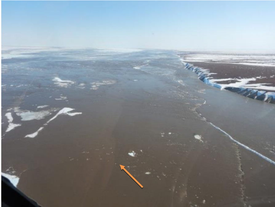
Figure 26. Measurement reach looking north on May 18, 2015. The Franklin Bluffs are on the right. Most of the flow is on the east (right) side of the channel, partially contained by a failing snow dike. Water is flowing over ice to the left (west) of the snow dike.
