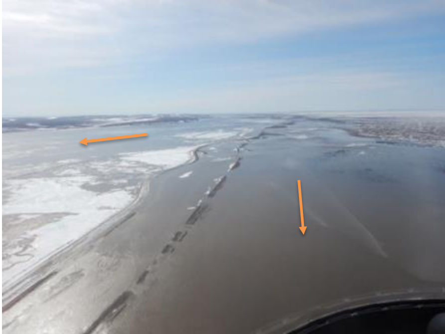
Figure B.7. Photo taken May 20, 2015, near Dalton Highway MP400, view south. Continued high water west (right) of the road and pipeline. Note completely submerged sections of road in this area. A Sagavanirktok River channel is at far left, and Franklin Bluffs are seen in the distance, upper left of center.
